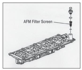
FIG 2: Valve Lifter Oil Manifold
