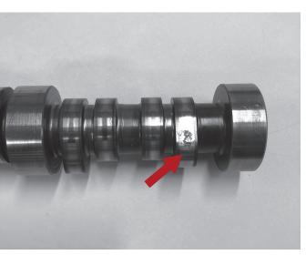
FIG 3: Camshaft Lobe Wear
