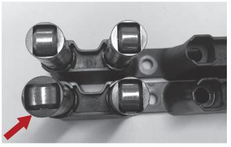
FIG 1: Worn Lifter Guide/Misaligned Roller
