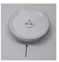
Detail of damaged plastic gear shown in Fig. 1
