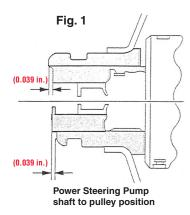
Some of the mentioned trucks produced prior to June 2004 may have an AC compressor/power steering pump mounting bracket and rear power steering mounting bracket machined slightly out of spec, resulting in a misaligned power steering pump. If this condition is present, the drive belt will be out of alignment with
