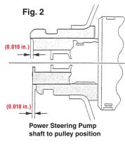
resulting in belt noises. The spec calls for the pulley to be flush with the end of the pump shaft. If the belt is not properly aligned with the pulley in this position, GM advises that the pulley should be repositioned on the pump shaft with a maximum variance of 0.010 inch from the end of the pump shaft (see Fig. 2). Notice how the pulley
