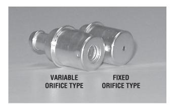
inch hole drilled in the bottom of the valve, providing a fixed flow rate. When servicing, technicians must be aware of the factory modification and be certain not to install the same type variable orifice valve that originally came on the vehicle. Doing so would reintroduce the performance condition that was corrected with the fixed orifice design.
